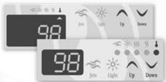
Use **Up/Down** arrow keys to regulate water temperature. Press and hold key to increase or decrease current water temperature setting. The temperature setting is displayed for 5 seconds to confirm your new selection. The "Set Point" indicator shows the desired temperature, NOT the current water temperature! Water temperature can be adjusted by 1°
