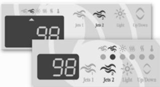
Press **Jets 2** to turn Pump 2/blower on. Pressing a second time turns Pump 2/blower off. A built-in timer turns Pump 2/blower off after 20 minutes, unless manually deactivated first. The "Jets 2" indicator lights up when Pump 2/blower is on.
