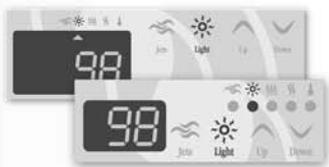
Press **Light** to turn light on. Press a second time to turn light off. The light turns off after 2 hours, unless it has been manually deactivated. The "Light" indicator is displayed when light is on.
