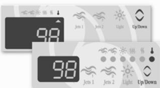
Use **Up/Down** arrow key to regulate water temperature. Press and hold key to increase or decrease current water temperature setting. The temperature setting is displayed for 5 seconds to confirm your new selection. The "Set Point" indicator shows the desired temperature, NOT the current water temperature!
