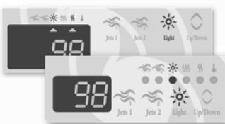
Press **Light** to turn light on. Press a second time to turn light off. The light turns off after 2 hours, unless it has been manually deactivated. The "Light" indicator is displayed when light is on.
