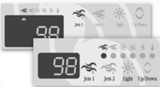
Press **Jets 1** to turn Pump 1 on. Press a second time to change Pump 1 speed. A third time turns Pump 1 off. A built-in timer turns Pump 1 off after 20 minutes, unless manually deactivated first. The "Jets 1" indicator lights up when Pump 1 is on.
