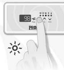
When the desired setting is displayed, press **Light** key again. The filter cycle will start. The "Filter" indicator lights up when a filter cycle is on.
