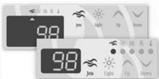
Press **Jets** to turn pump on. Press a second time to change pump speed. A third time turns pump off. A built-in timer turns pump off after 20 minutes, unless manually deactivated first. The "Jets" indicator lights up when pump is on.
