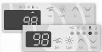
When water temperature is 1°F (0.5°C) lower than Set Point, the heater will automatically turn on until water temperature reaches Set Point plus 1°F (0.5°C).
