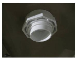
To install the return fitting, you need to un-thread the retaining nut from the fitting. Insert the threads through the prepunched hole from the inside of the pool and tighten the retaining nut to the back of the fitting. Do not over tighten this nut.
