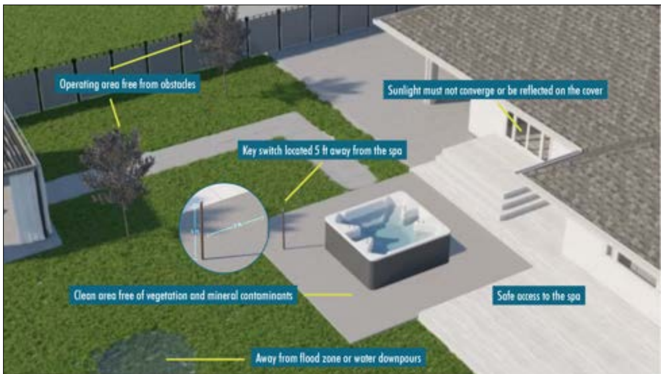
FIGURE 2: PREPARATION FOR THE INSTALLATION
