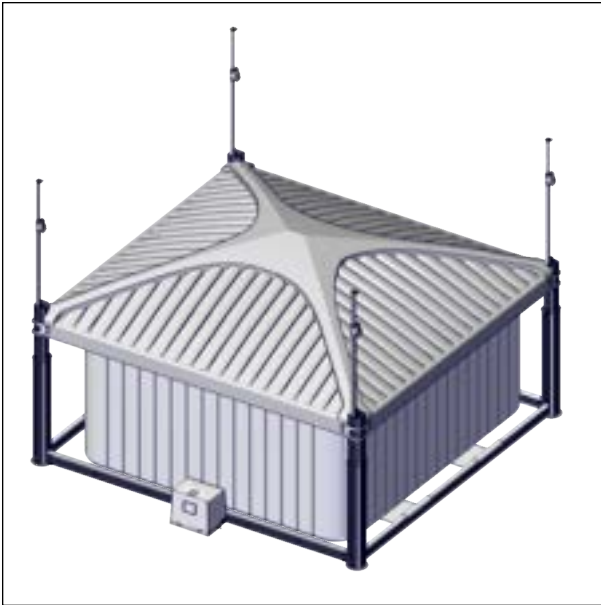
FIGURE 85: SPRAY GREASE ON SLIDING PARTS AND MECHANICAL COMPONENTS OF EACH JACK
