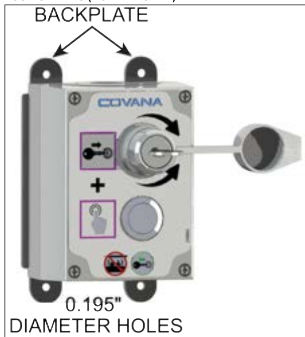
FIGURE 50: FASTEN BACKPLATE OF KEY SWITCH WITH FOUR SCREWS (NOT INCLUDED)
