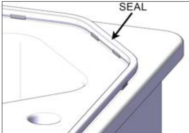
FIGURE 57: INSERT CONNECTOR IN BOTH ENDS OF THE SEAL
