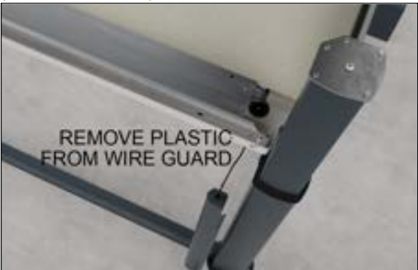
FIGURE 28: REMOVE WIRE GUARD FROM INNER SHELL (LET IT HANG DOWN)
